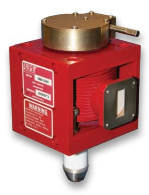
A magnetron is a high power microwave oscillator in which the potential energy of an electron cloud near the cathode is converted into RF energy in a series of cavity resonators. The VMX3045 magnetron delivers high peak and average RF power for use in medical or industrial applications.
